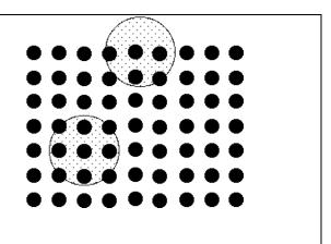
As temperature increases, the atoms in a solid vibrate more, and reduce the cohesive force binding the atoms. The surface energy depends on the net inward cohesive force and so surface energy decreases with increasing temperature. The surface energy for many metals (e.g. Ag, Au, and Cu) goes down by about 0.5 mJ.m<sup>2</sup>.K<sup>-1</sup> with increasing temperature. Water goes down by about 160 mJ.m<sup>2</sup>.K<sup>-1</sup>.
